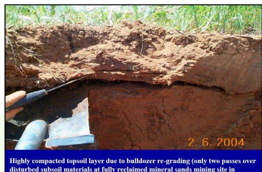
Highly compacted topsoil layer due to bulldozer re-grading (only two passes over disturbed subsoil materials at fully reclaimed mineral sands mining site in Dinwiddie County (details later). Can only be remediated via deep tillage. Most revegetation species need at least 6" to > 18" of effective rooting.
